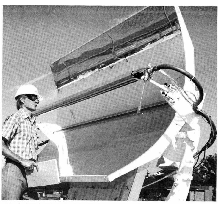
IN 1980, the Photovoltaic Advanced Systems Test Facility became operational. It has capability for testing a variety of photovoltaic collectors and analyzing test data. Dan Pritchard (4721) stands near an Acurex collector under test.
